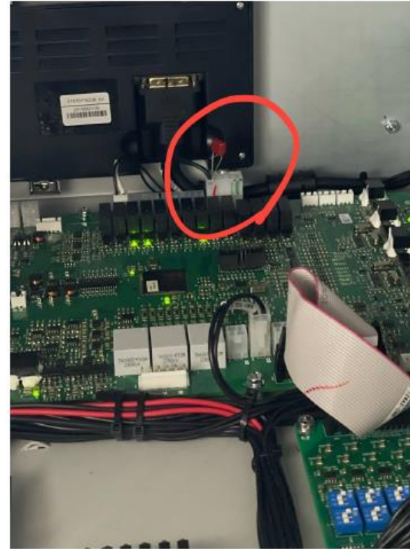
Figure 17. Installation of the film capacitor inside the XXXXXXXXXX
