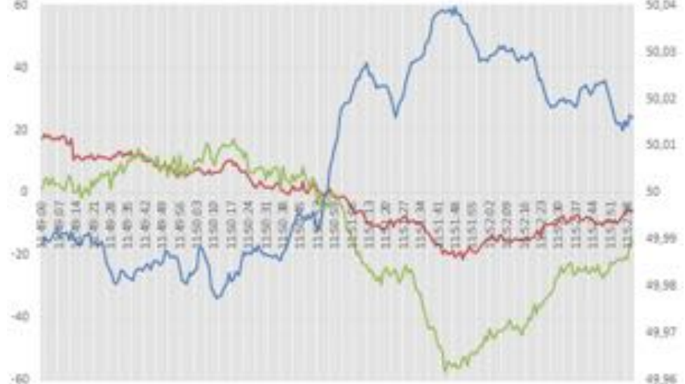
FCR after outage of 88 MW (3 rd test)
