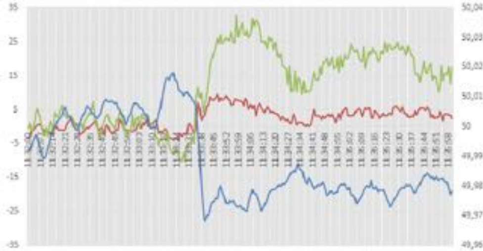
FCR after outage of 88 MW (3 rd test)
