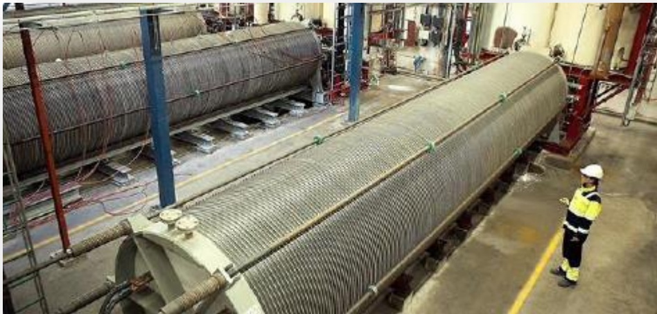
2.25 MW alkaline stack
