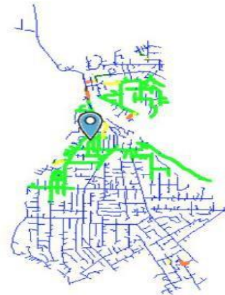
Peak 2034 COM Power Flow After Mitigation
