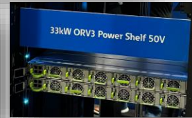
Two 33 kW Power shelves each with 6 PSUs (2 x 6 x 5.5 kW)
