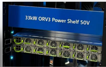
Two 33 kW Power shelves each with 6 PSUs (2 x 6 x 5.5 kW)
