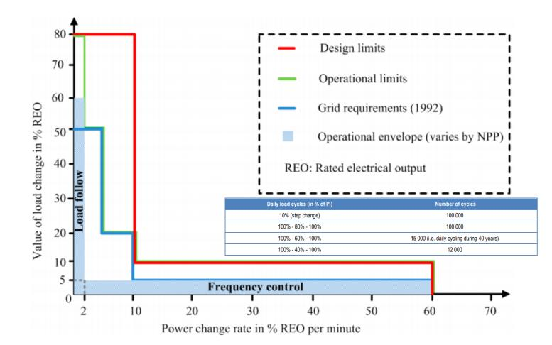
German pressurized water reactor flexibility requirements and designed capabilities (courtesy of H. Ludwig, AREVA GmbH)
