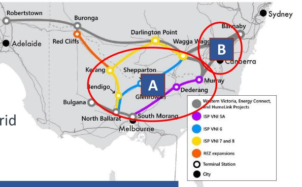
A. New 500kV/330kV Infrastructure is required to increase transfer capacity between Victoria and NSW. GETs allows you to fully utilitise the capacity delivered by new infrastructure. B. New 500kV Infrastructure to connect Snowy Hydro plus other REZ to Sydney adding GETs north of Bannaby future proofs the overall solution by unblocking a downstream constraint.
