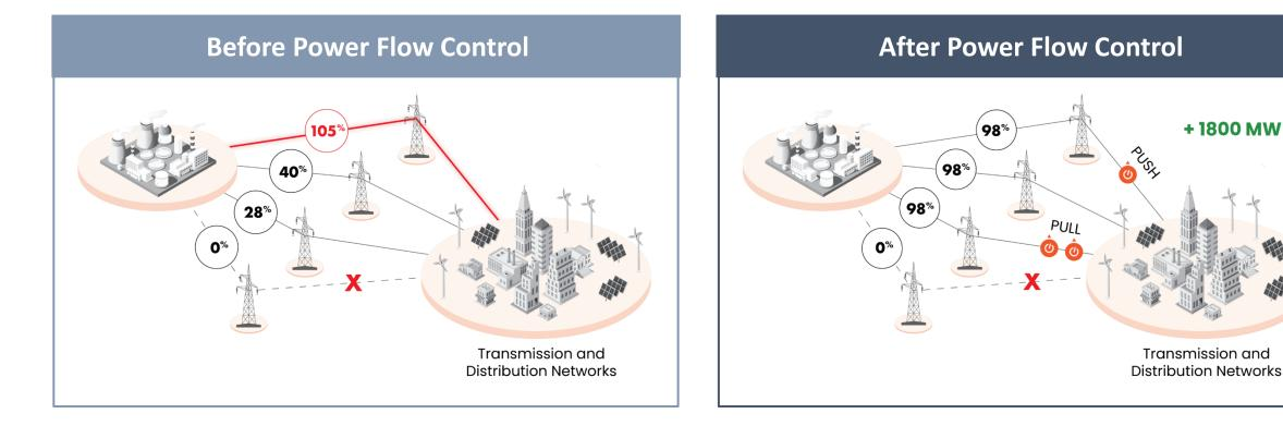
Power flow control enables the efficient operation of the existing transmission grid
