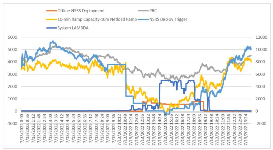
\*Triggers for OFFLINE Non-Spin Deployment: (1) (High Ancillary Service Limit (HASL) – Gen – Intermittent Renewable Resource (IRR) Curtailment) – (30-minute net load ramp) < 0 MW (2) Physical Responsive Capability (PRC) < 3200 MW and not expected to recover within 30 minutes without deploying reserves
