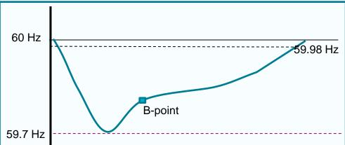
*B*-point (settling frequency) is determined using dynamic simulations/studies that are run at varying inertia levels. In every simulation, a single mediumsize unit is tripped offline such that the C-point (frequency nadir) is stays just above 59.7 Hz\*.
