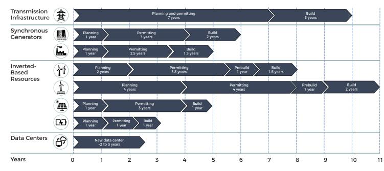
Timelines for grid infrastructure are not aligned with those for large load development, creating bottlenecks for grid supply of electricity. SOURCE: ADAPTED FROM S&P GLOBAL.
