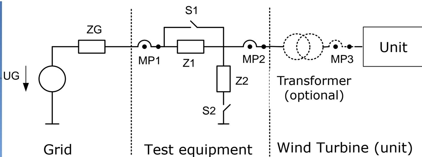
Measurement setup according to IEC 61400-21 / FGW TG3
