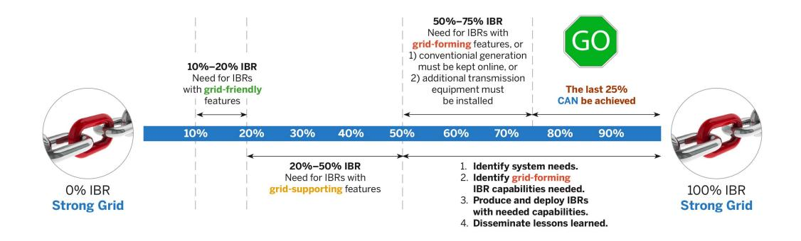
Deploying grid-forming capabilities from IBRs themselves is cheaper and faster than adding new transmission assets, which would require additional investment and take much longer to build.
