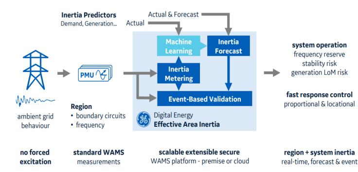
Source: NASPI Working Group Meeting, <u>GE Effective Area Inertia: Stability</u> <u>Challenges, PMU-Based Metering & Machine Learning Forecasting</u> • Uses "ambient" changes in system frequency
