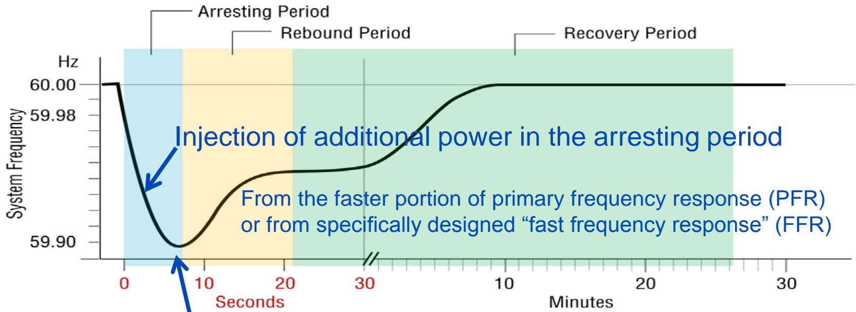
Goal is to establish the “nadir” (minimum frequency point) before reaching under frequency load shedding (UFLS)
