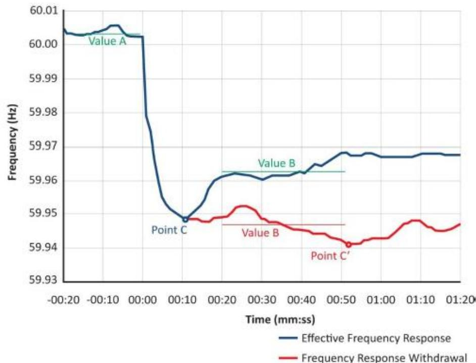
**A to B frequency response** captures the effectiveness of primary frequency response in stabilizing frequency following a large frequency excursion. This Measure is the conventional means of calculating frequency response as the ratio of net MW lost to the difference between Point A and Point B frequency values.
