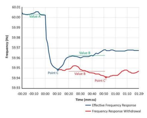
A to B frequency response captures the effectiveness of primary frequency response in stabilizing frequency following a large frequency excursion. This Measure is the conventional means of calculating frequency response as the ratio of net MW lost to the difference between Point A and Point B frequency values.
