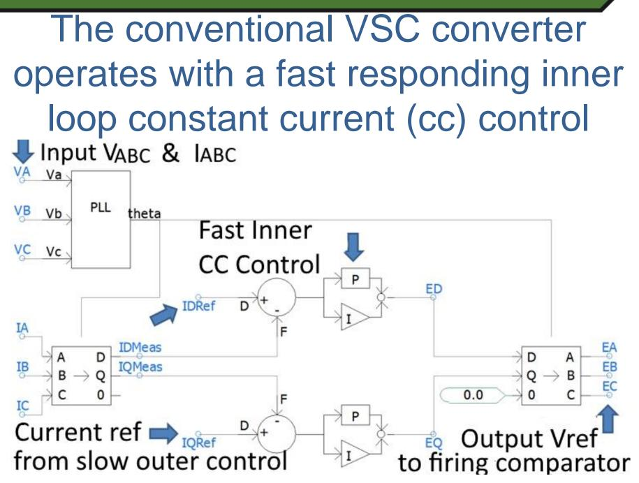
What is a fast VSC voltage source instead of the fast current source of regular VSC converters?
