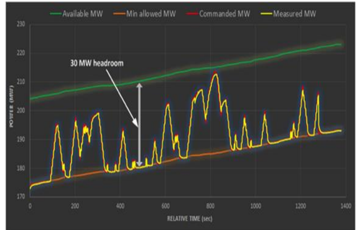
NREL/FirstSolar/CAISO experiment: 300-MW plant following Automatic Generator Control (AGC) signal
