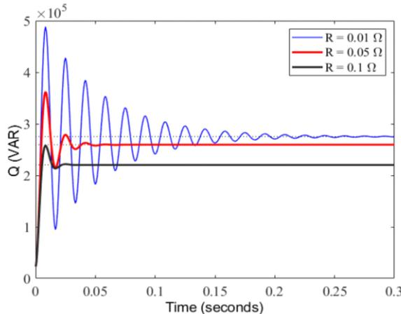
$$\left. \frac{Q(s)}{V_m(s)} \right|_{\theta(s)=0} = \frac{Q_0}{V_1} - \frac{3}{2} V_1 \cdot \frac{\omega_1 L}{(R + sL)^2 + (\omega_1 L)^2}$$
