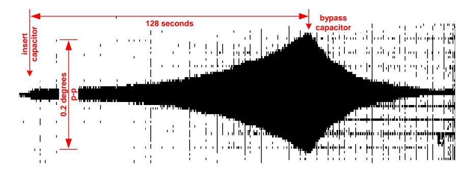
Measured SSR Instability: series capacitor inserted and bypassed after 128 seconds.
