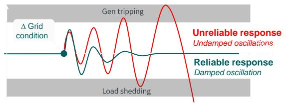
*Ex*: Sub-synchronous resonance (SSR) can break shafts
