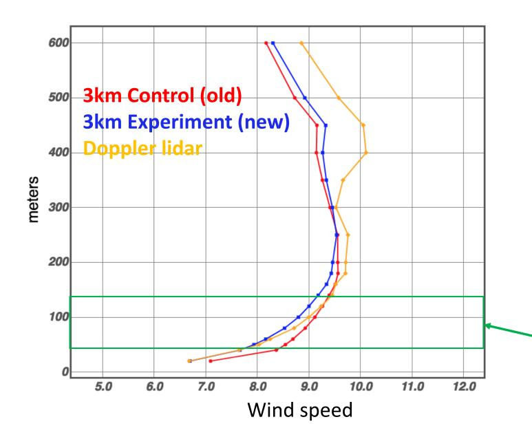
Average of all wind speed profiles with wind directions at 80 m AGL between 225 and 315 degrees during **July 2016**.
