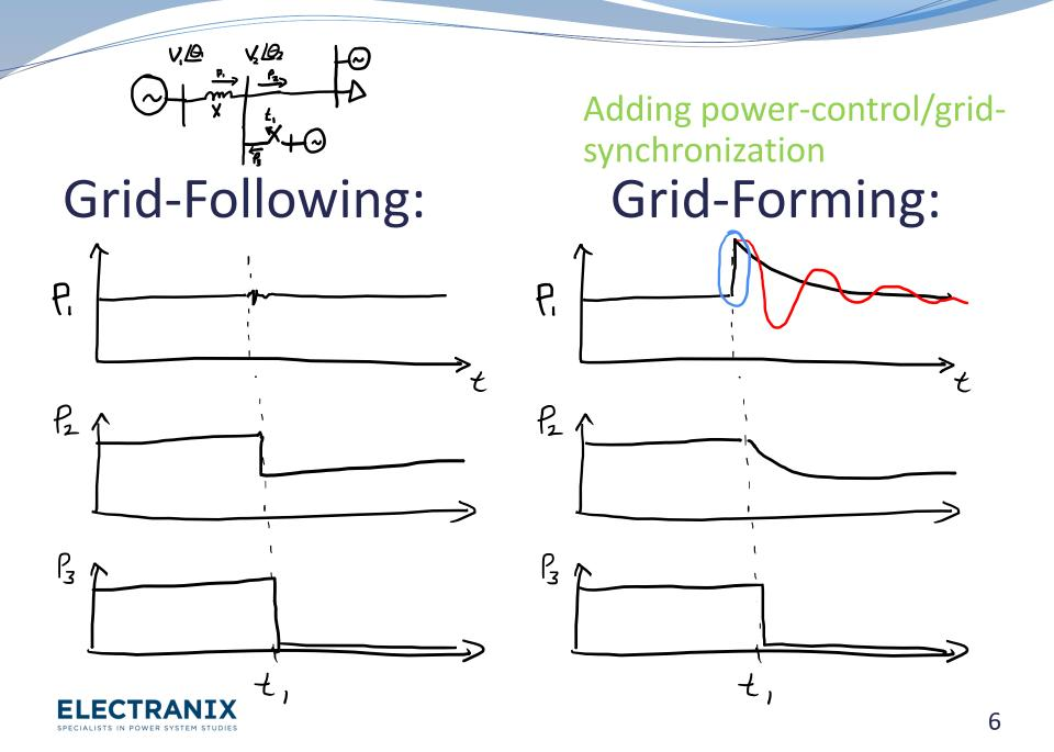
Adding Power Control/Grid Synchronization Adding frequency-droop control
