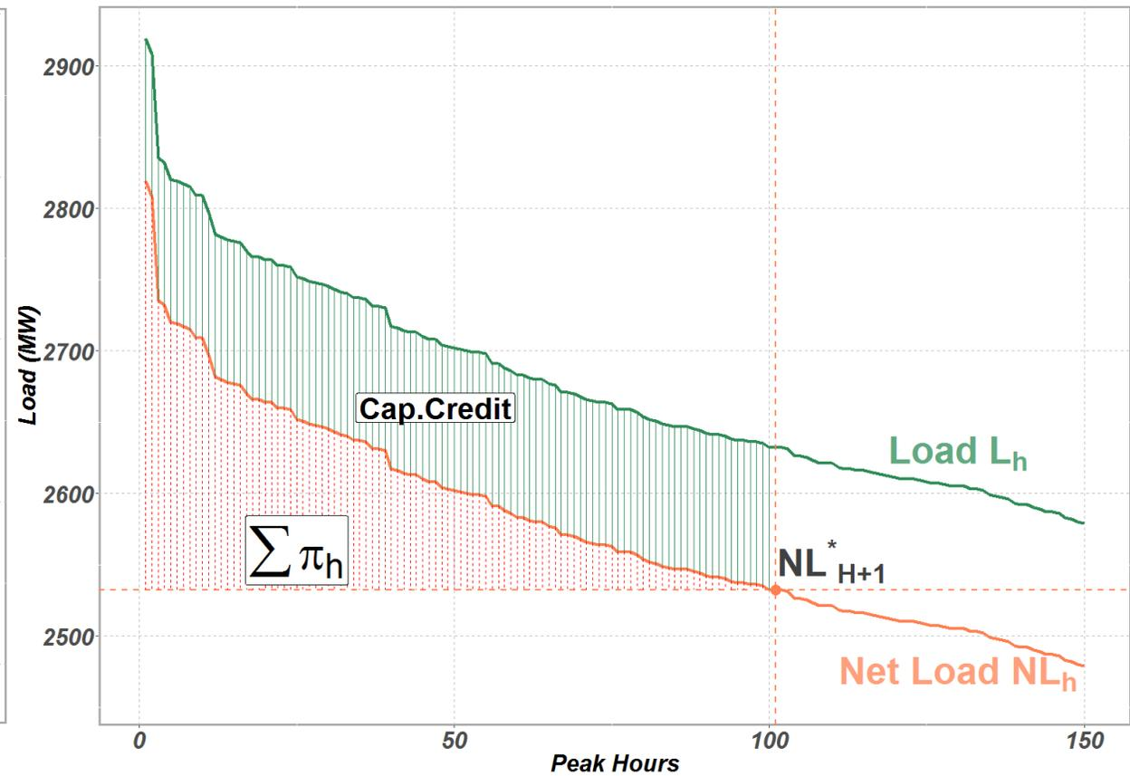
Define capacity credit similar to NREL's "Resource Planning Model": difference of the highest peak load hours and highest peak net load hours. Use a simple linear model to find the storage dispatch that maximizes this capacity credit.
