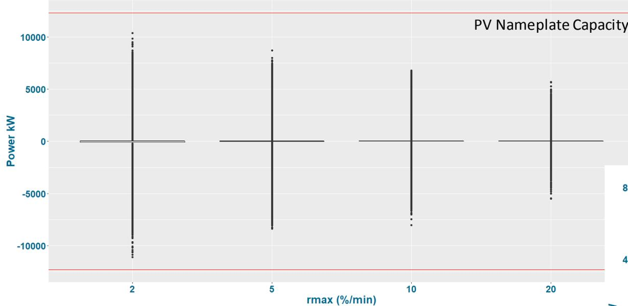
Battery Power: Charge and Discharge per minute for Talla year 2017
