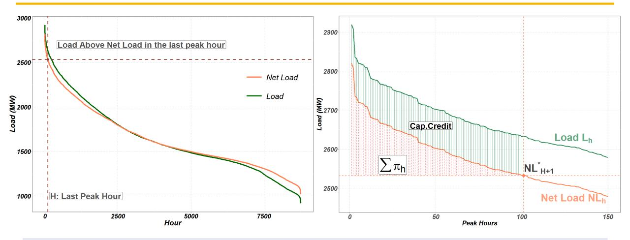
Define capacity credit similar to NREL's "Resource Planning Model": difference of the highest peak load hours and highest peak net load hours. Use a simple linear model to find the storage dispatch that maximizes this capacity credit.
