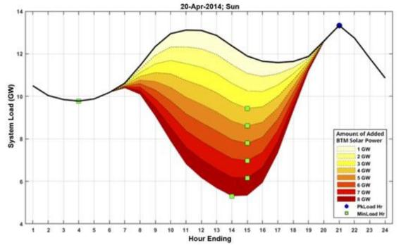
The integration of solar generation complicates the ability of dispatchable generation to track net load.
