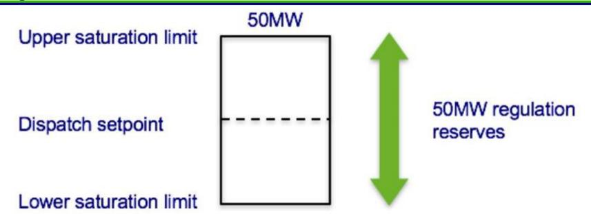
Regulation Reserves: Power capacity available during normal conditions to assist in active power balance and to correct any imbalances that requires a fast, real-time, automatic response.
