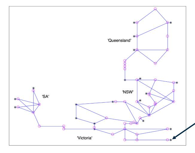
Apply 3-phase faults on main transmission nodes (for which original system remains stable)
