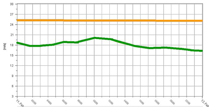
**1 wind speed forecast in the unit [m/s]**, which is a mean forecast from 75 ensemble members and smoother than a typical deterministic forecast. **Additionally, you see a reference line for the 25m/s threshold reference value** for high-speed shutdown or also sometimes called cut-off wind speed threshold.
