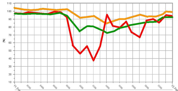
**3 independent deterministic wind power forecasts in the unit [% of installed capacity]** based on 3 different NWP (numerical weather prediction) models
