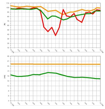
3 independent deterministic wind power forecasts in the unit [% of installed capacity] based on 3 different NWP (numerical weather prediction) models
