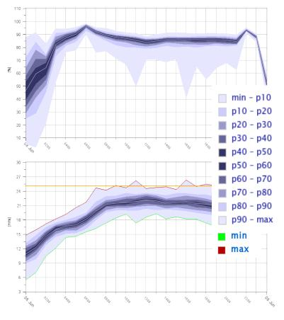
9 wind power percentiles (P10..P90) and a mean (white line) in the unit [% of installed capacity] generated from 75 NWP forecasts of a multi-scheme ensemble prediction system.
