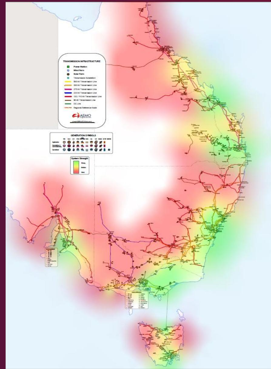
Connections in areas with low system strength are driving installation of synchronous condensers by developers
