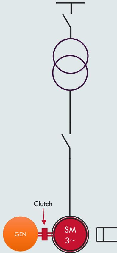
Hybrid synchronous condenser with a FACTS controller, e.g. STATCOM
