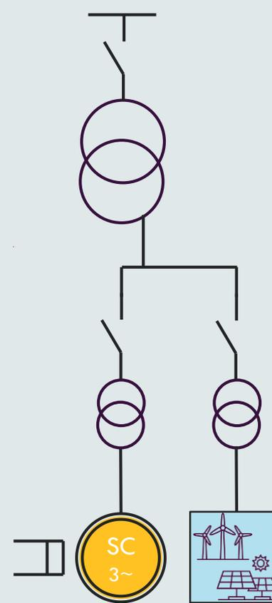
Synchronous condenser in a different location to the inverter-connected generator
