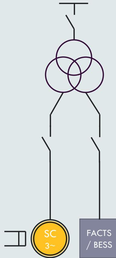
Synchronous condenser co-located with inverter-connected generator
