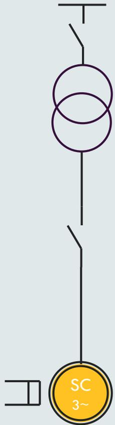
Conventional generator operating as a condenser (with or without clutch)
