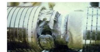
Failed Rotor at Mohave
