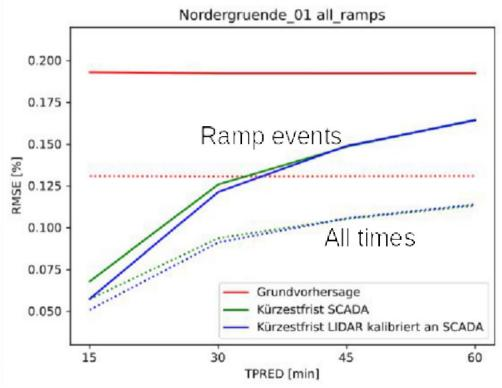
LIDAR-assimilated forecasts perform better in shortest-term, especially during ramp events
