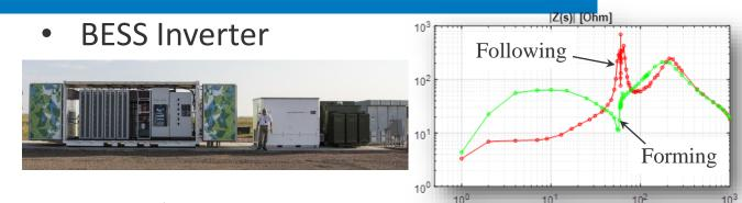
• Impedance measurements can quantify different aspects of gridforming ability
