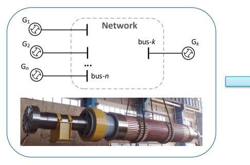
Traditional generators: create 50 Hz AC from a rotating electro-magnet. Dynamics are described by well-known physics equations
