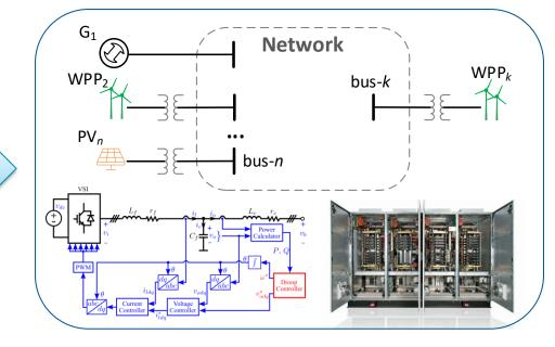
Inverter-based resources (IBR): dynamics are set by control software and behaves differently as traditional synchronous generators.
