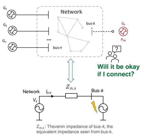
Short-circuit capacity (SCC):  $\operatorname{SCC}_{k} = \frac{|V_{s}|^{2}}{|Z_{th,k}|}$
