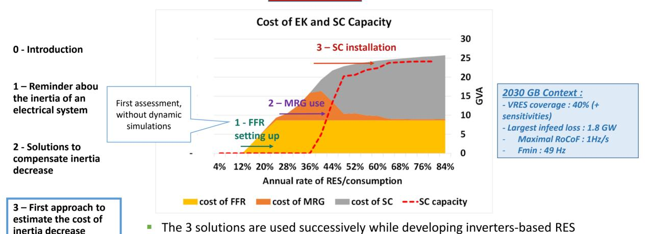
SC installation enables to limit the KE costs
