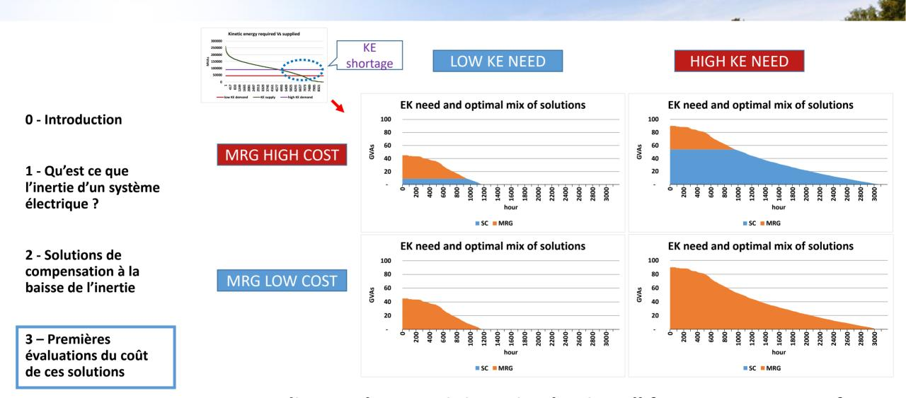
Depending on the case, it is optimal to install from 0 to 54 GVAs of SC (30 GVA of SC)
