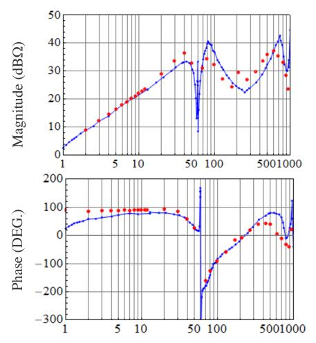
Blue: Measurements of 4-MW DFIG Red: OEM PSCAD model
