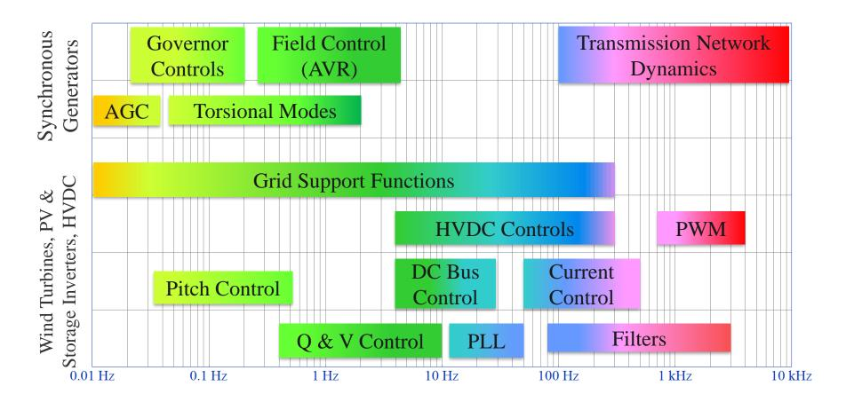
• Power electronics-based generation and transmission technologies have increased control interaction problems
