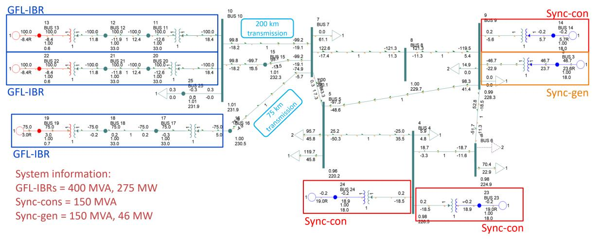
Study objective: To allow retirement of synchronous condensers and generator from the load centers, where to place a GFM device and what should be its rating?
