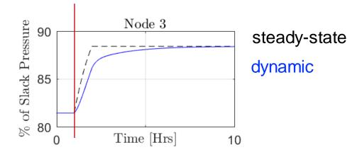
It takes a LONG time for the steady-state solution to settle down, more than 5h!
