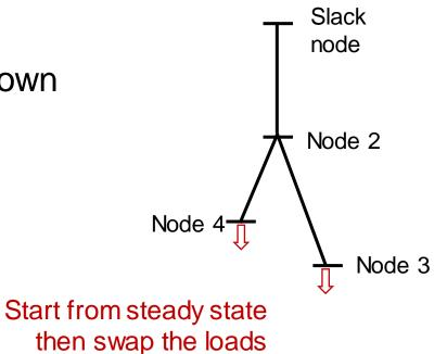
Steady-state gas system modelling: ------Assume that system dynamics have time to settle down
