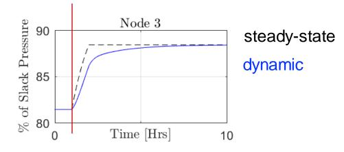
Steady-state gas system modelling: ------Assume that system dynamics have time to settle down
