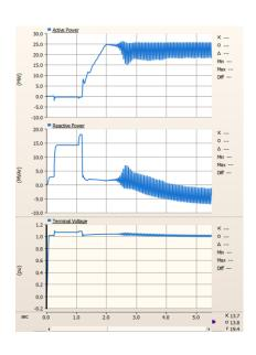
• IBR plant is unstable – confirmed by time-domain simulations (17.4 Hz)
