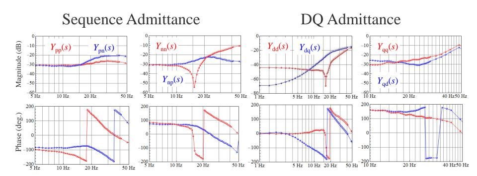
• Severe resonance at 17 Hz in  $Y_{dd}(s)$
