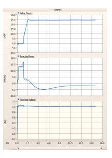
• IBR plant is stable with low stability margin – Plant still has highly underdamped resonance mode, but it will not excite oscillations in the absence of a disturbance
