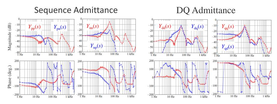
•  $Y_{dd}(s)$  shows damped of resonance near 18 Hz.
