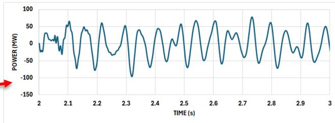
GFL BESS providing SSR damping control
