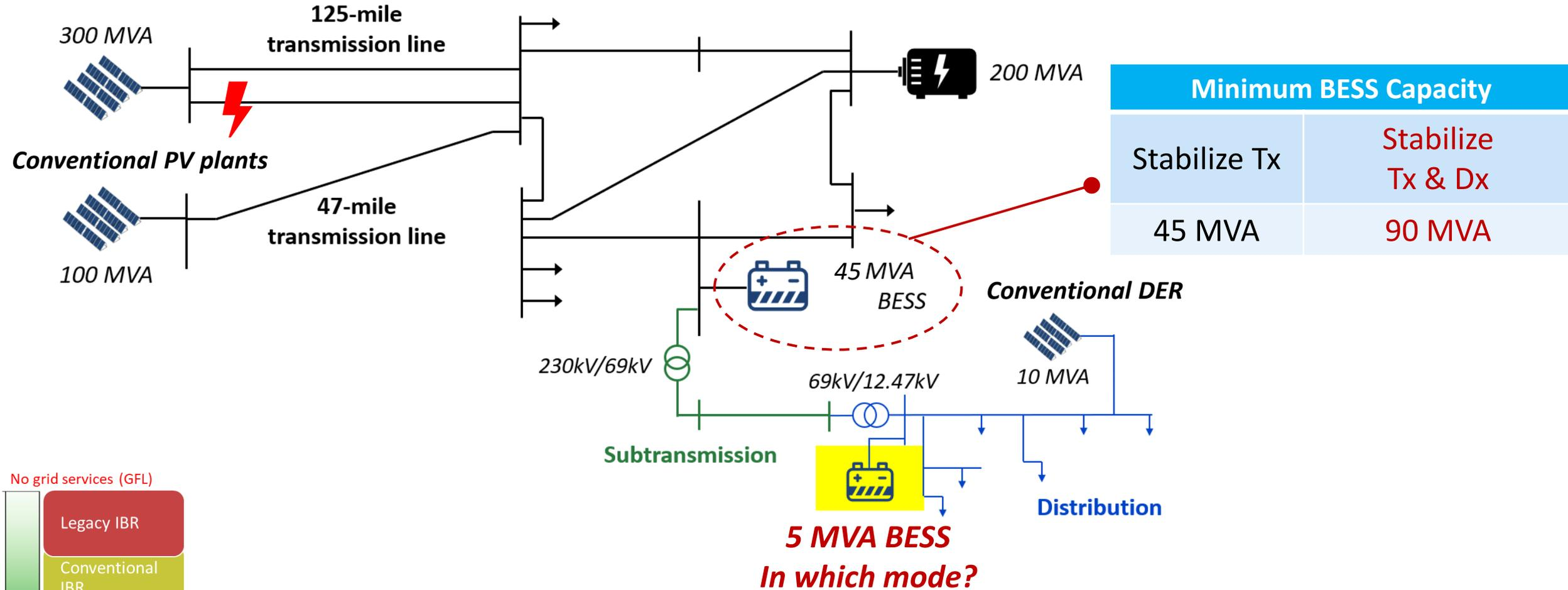
*If a 5MVA BESS is installed at the Dx substation, does it benefit system stability by operating in which mode?*
