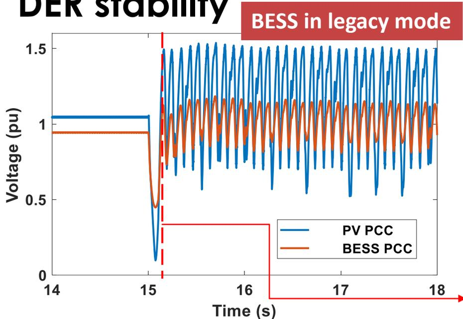
*The 10MVA DER would be tripped if IEEE 1547-2018 trip settings are activated*
