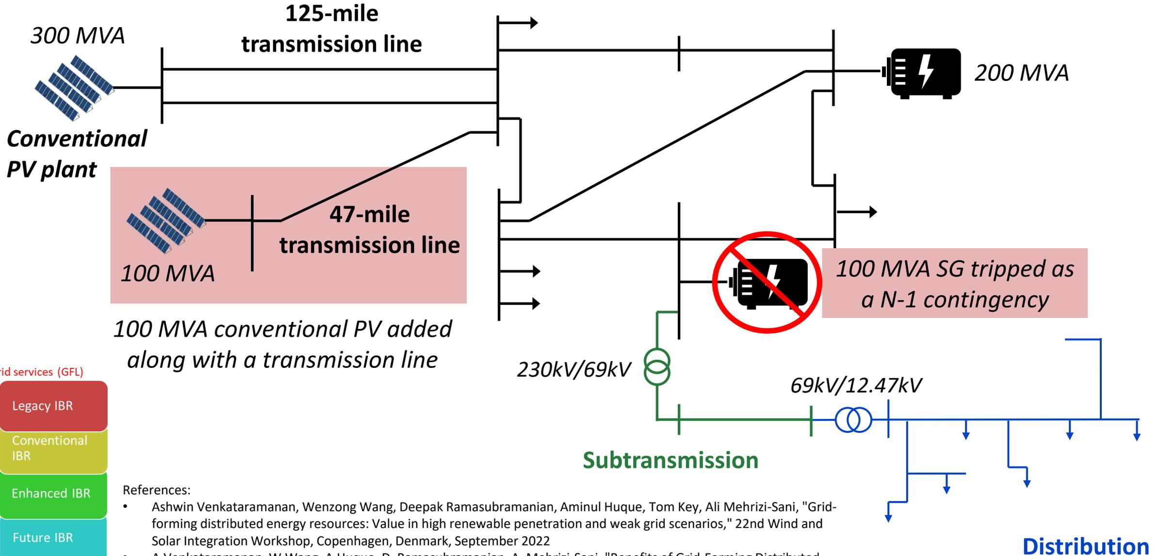
100 MVA conventional PV added along with a transmission line
