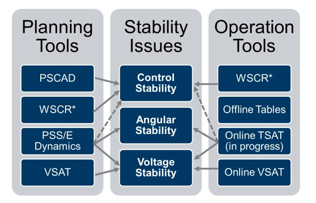
\* WSCR (weighted short circuit ratio) is used to identify the system strength of an area with multiple IBRs. Detailed PSCAD studies are required to validate the adequacy of WSCR application and its threshold for weak grid identification.
