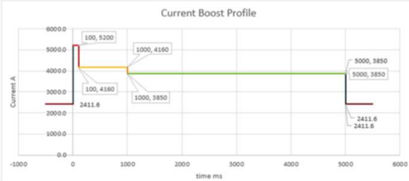
Inverter level current boost profile
