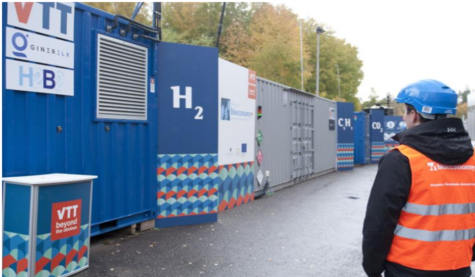
Plug Power Electrolyzers. Hydrogen from electrolysis combined with CO 2 captured from air/industrial sources/etc... to produce Biomethane & Biofuels
