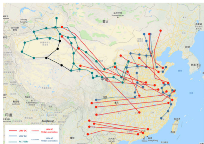
Figure 3. The ultra high voltage transmission system in China in 2018.
