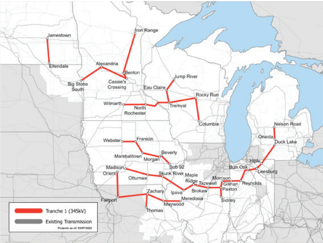
FIGURE 4 Map of Proposed MISO Long Range Transmission Planning Tranche 1 Transmission Upgrades
