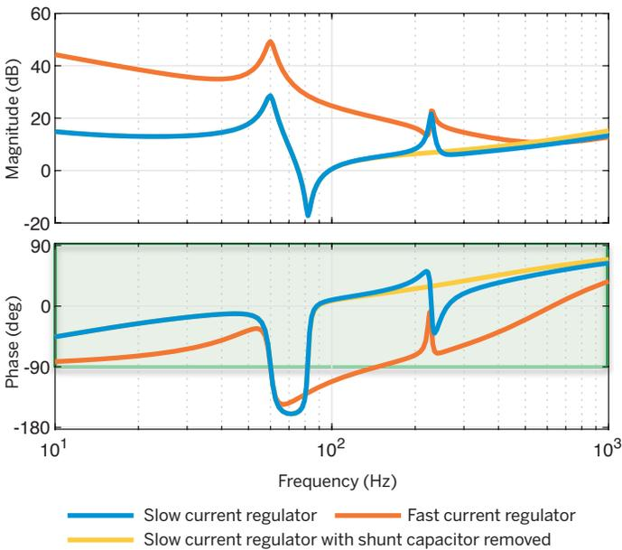
The magnitude and phase of the combination of a PV inverter and the host grid show a supersynchronous resonance at about 80 Hz. Two variations (fast and slow) in the current regulator shift the phase somewhat, but both remain outside of the green positive damping band of  $\pm 90^\circ$ . A higher frequency positively damped resonance at about 220 Hz is due to a nearby shunt capacitor, which disappears when it is removed (yellow line).
