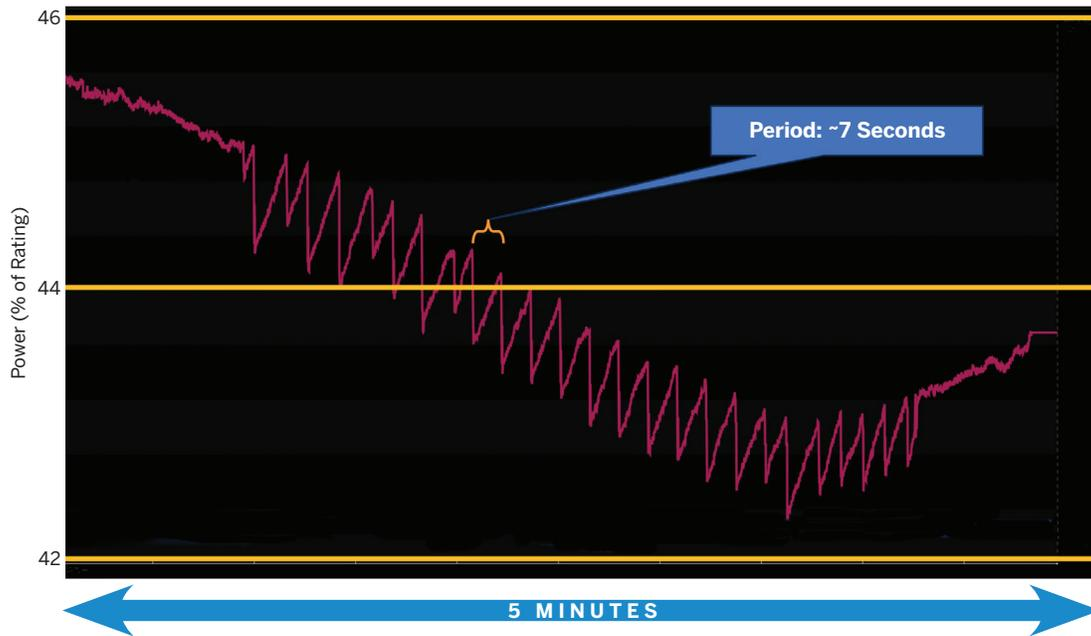
The sawtoothed behavior of active power shows a limit cycle of about 7-second periodicity, pointing to a control pathology in which a discrete threshold is hit repeatedly. The systemic conditions that create this tuning come and go, as can be observed at the beginning and end of the measurement sample.
