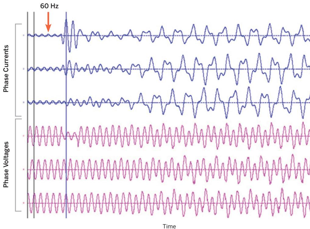
Field measurements of a wind plant entering into subsynchronous oscillations after being tripped on fault clearing to a radial connection through a transmission series capacitor. Oscillations are at about 25 Hz and were of sufficient magnitude to damage equipment. Mitigation included relays, reduced compensation, and addition of damping controls.
