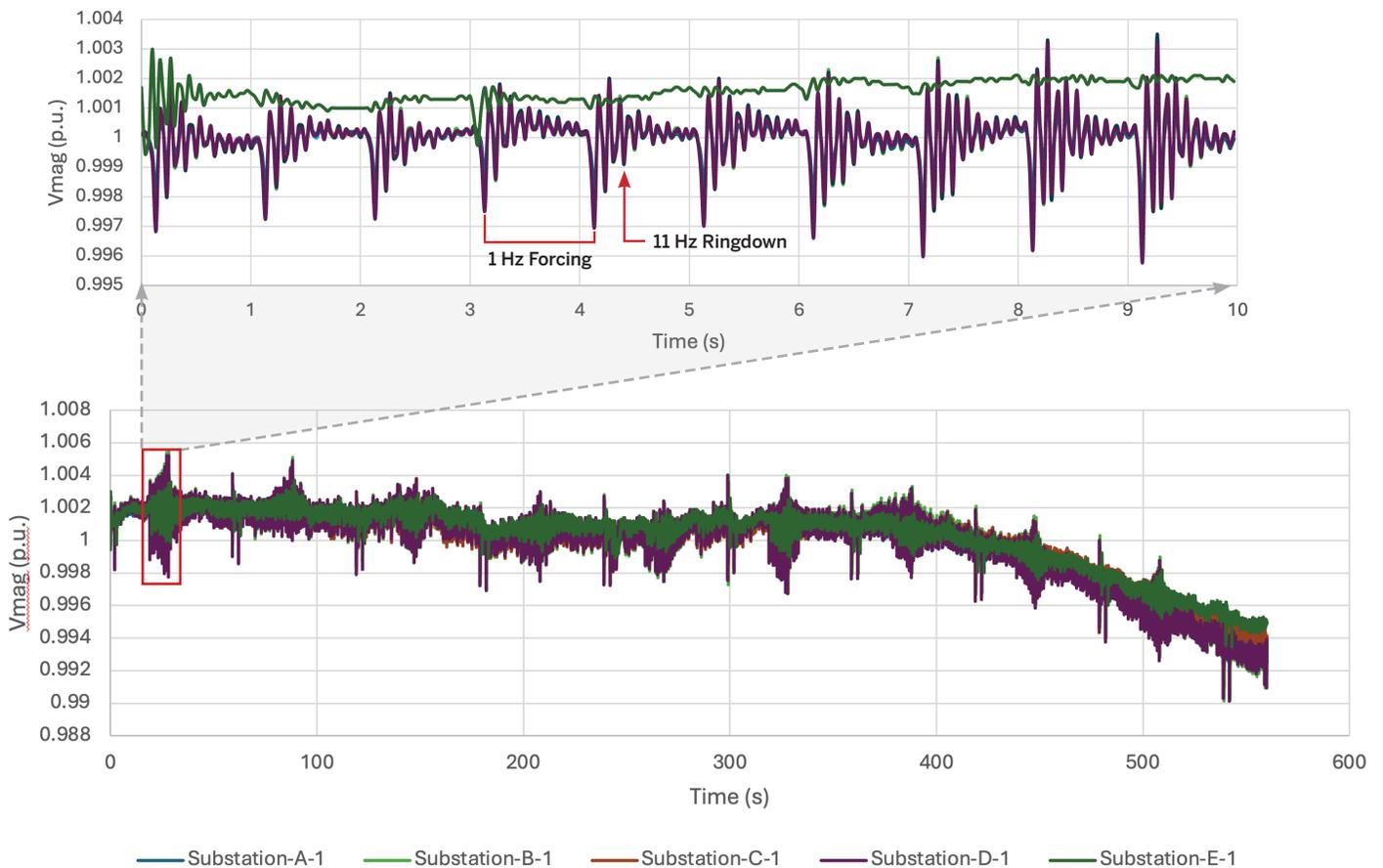
Field measurements of forced oscillations occurring at 1Hz that are driven by a misbehaving load. A positively damped system resonance at 11Hz is stimulated by each discrete forcing event. The bad actor was found using an oscillation localization tool. Some substation plots are behind others and thus not visible.
