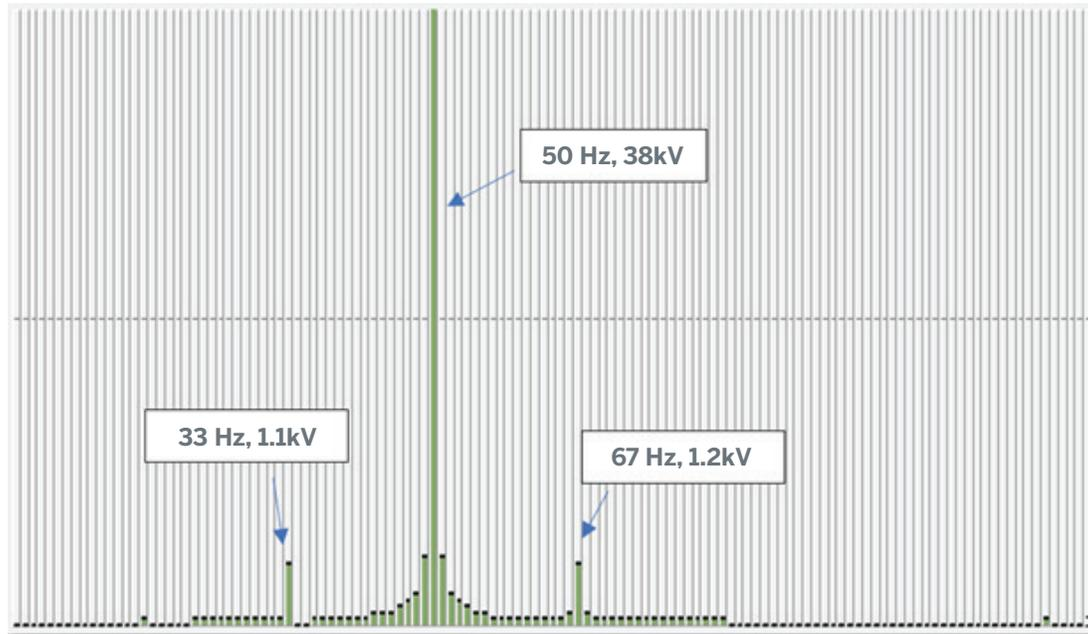
**Fast Fourier transform (FFT) of a 50 Hz voltage being modulated at 17 Hz. The FFT sidebands at  $\pm$  the modulation frequency around fundamental frequency are characteristic of modulated oscillations. The diagnostician is not concerned with 33 and 67 Hz phenomena per se.**
