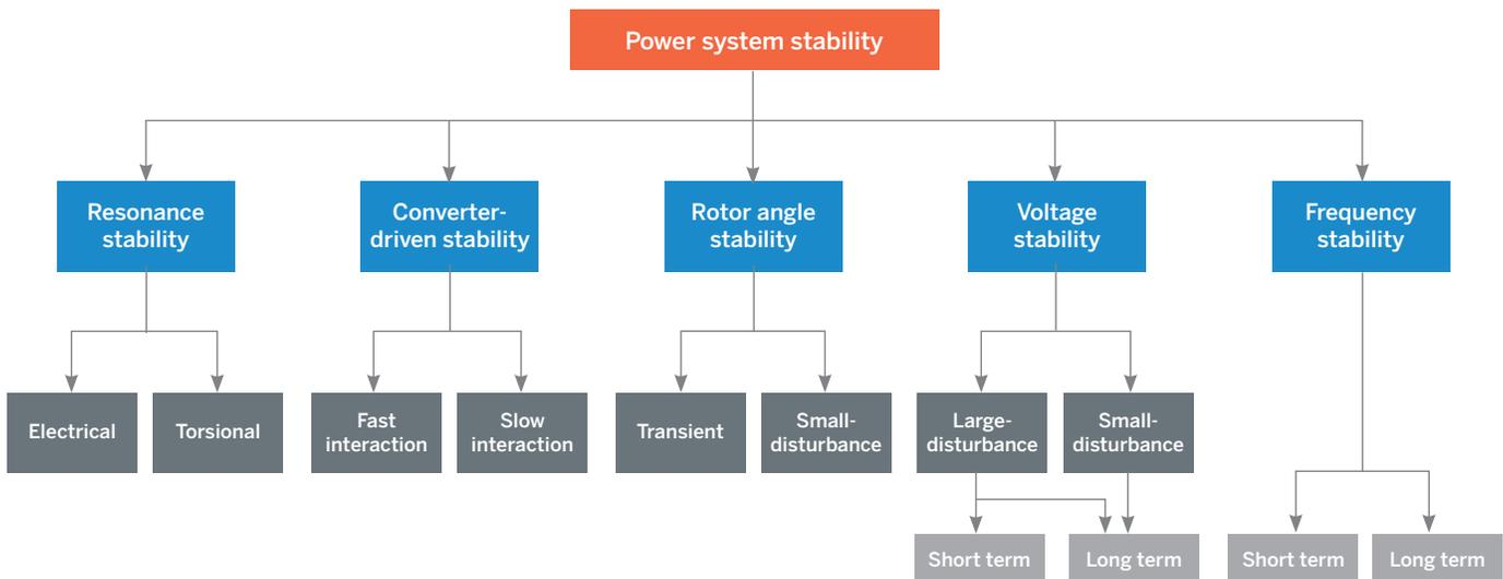
On the right-hand side, the figure shows the familiar classification of power system stability. In the recent version of stability definitions, two additional categories were introduced, resonance stability and converter-driven stability, to recognize stability phenomena that are becoming more prominent with growing shares of IBRs. For diagnosis of oscillatory problems, this guide has adopted a modified taxonomy.
