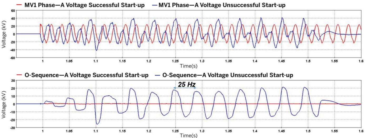
On-site measurement of an SVC being driven into 25 Hz ferroresonance during start-up (blue traces). Note that the instability manifests in the zero sequence voltage. Increasing the size of the surge capacitor mitigated the problem and allows for successful start (red traces).
