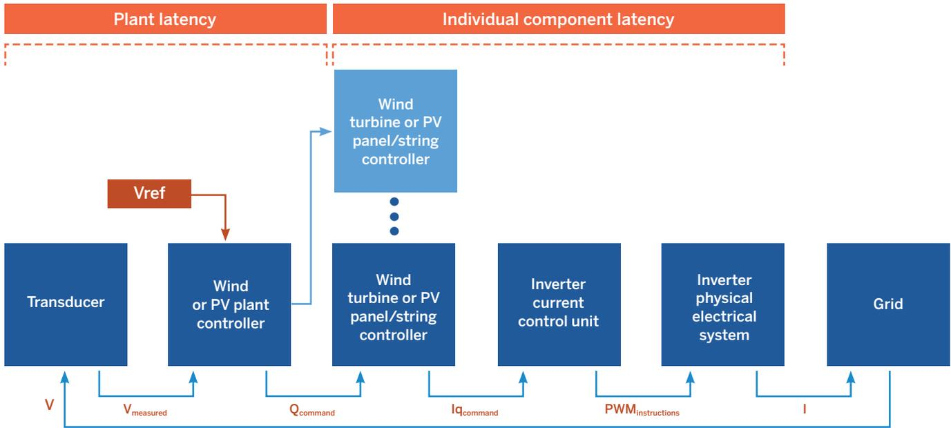
Information flow in a representative wind or solar PV plant, showing the various data transfer and processing steps that can add latency in controls. Plant-level controls, on the left, are physically separate from individual IBR elements, on the right. Processing (within the boxes) and transmittal (arrows between) may each contribute to delays.
