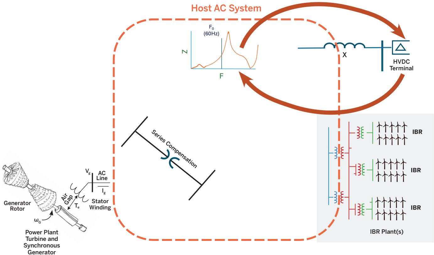
This diagram showing the main components of a power system highlights interactions between the host network and HVDC (as shown by the red arrows). The thumbnail plot of impedance vs. frequency depicts the frequency-dependent nature of the network, which is a key element in creating conditions susceptible to oscillations due to this type of interaction.
