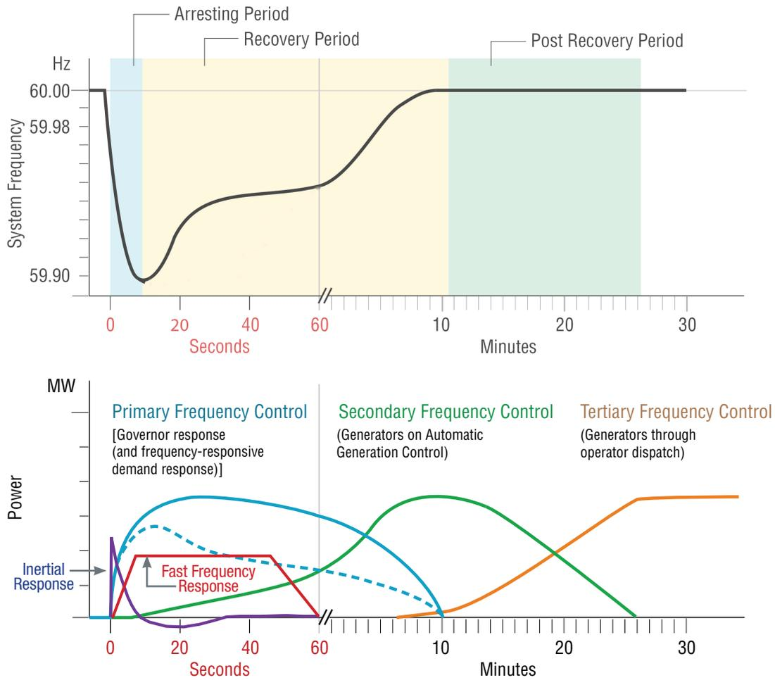
This is the figure widely used by NERC showing three distinct periods following a loss-of-generation event, and frequency control services that align with those periods. Inertial response and fast frequency response have been added to the figure. The five services all have characteristics that can lead to oscillations. The temporal overlap between services also creates the potential for oscillatory interaction between them.
