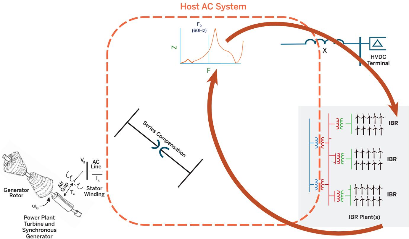
This diagram showing the main components of a power system highlights interactions between IBR plants and the host network (as shown by the red arrows). The thumbnail plot of impedance vs. frequency depicts the frequency-dependent nature of the network as viewed from different nodes or points of interconnection, which is a key factor in establishing the frequency and damping of oscillatory interactions with IBRs.
