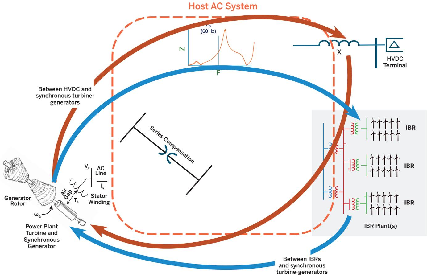
This diagram showing the main components of a power system highlights interactions between HVDC and synchronous turbine-generators (as shown by the red arrows) and between IBRs and synchronous turbine-generators (as shown by the blue arrows). This type of oscillation is specific to torsional interaction with inverters that neither is dominated by, nor requires the existence of, series compensation. This is “old school” HVDC SSTI, often referred to as simply “SSTI.”
