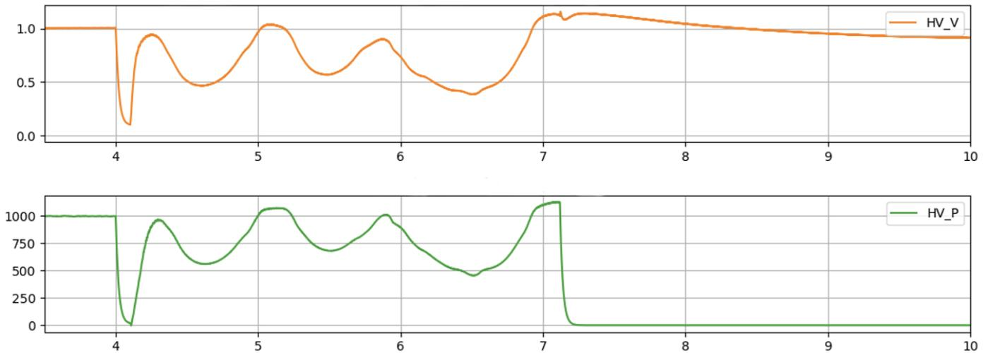
This is an example EMT simulation in which a grid-following resource is exporting power at a point near the nose of the post-fault PV curve. The system voltage (orange trace) and active power (green trace) exhibit unstable 1 Hz oscillation, ending in loss of synchronism as the voltage control fails to reestablish control. The behavior is highly nonlinear and would resist successful diagnosis using only state-space methods.
