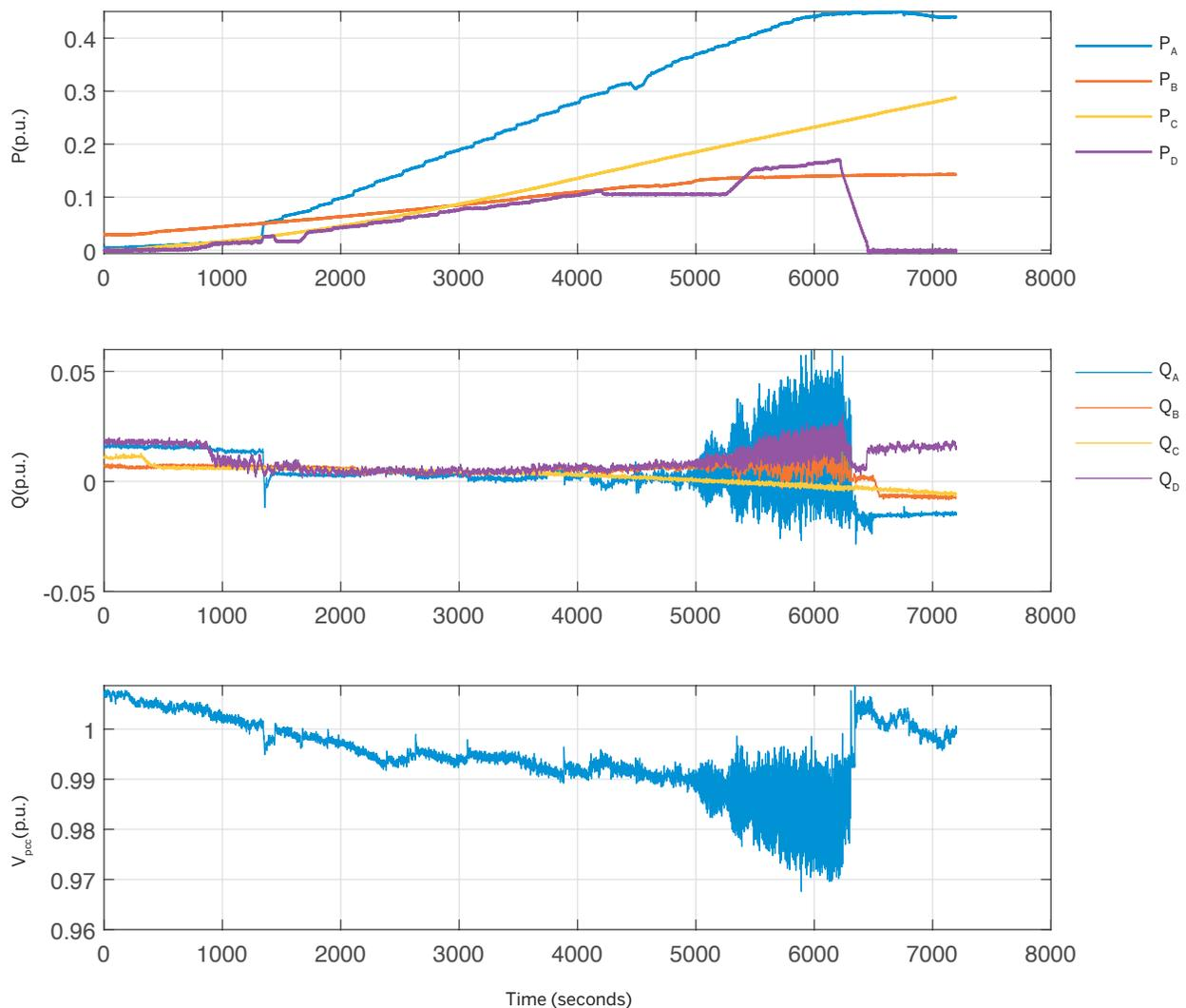
Active power of a large solar PV plant with four separate measurements is shown increasing over about 2 hours. Voltage oscillations driven by swings in reactive power stemming from excessive delays start at the power level reached at about 5000 seconds, and continue to grow as the system is stressed by approaching the nose of the PV curve for this point in the host system. Elements of the plant begin to trip at around 6300 seconds.
