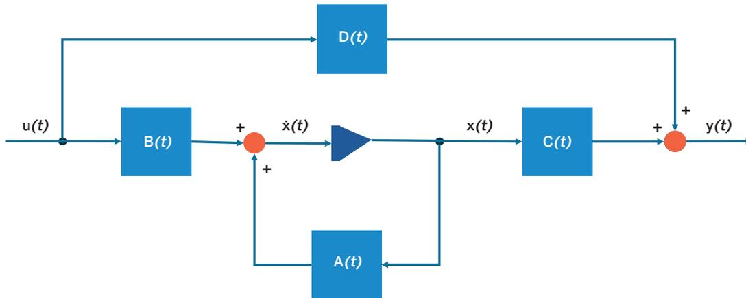
General state-space input/output block diagram from standard linear control theory. “A” represents the state matrix that defines the relationship between state variables, “B” represents the relationship between control inputs and state variables, “C” represents the relationship between state variables and measurable quantities, and “D” represents algebraic impacts of control inputs on measurements.
