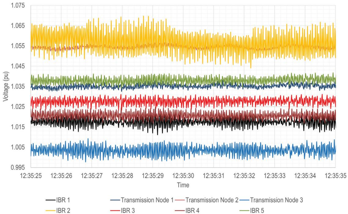
**Field measurements showing the voltage at five solar PV installations in relatively close electrical proximity oscillating in the 15-20 Hz range. There is some phase coherency between them, but it is imperfect, suggesting that they are interacting with each other as well as the host system. Inspection revealed a close correlation between oscillations and low irradiance conditions.**
