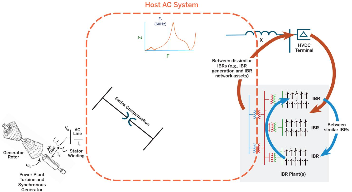
This diagram showing the main components of a power system highlights interactions between IBRs (e.g., IBR plants and HVDC) (as shown by the red arrows) or between different IBR plants which might be in close electrical proximity (as shown by the blue arrows). The interaction of different high-bandwidth controllers typical of these devices creates a variety of mechanisms for creating oscillations.
