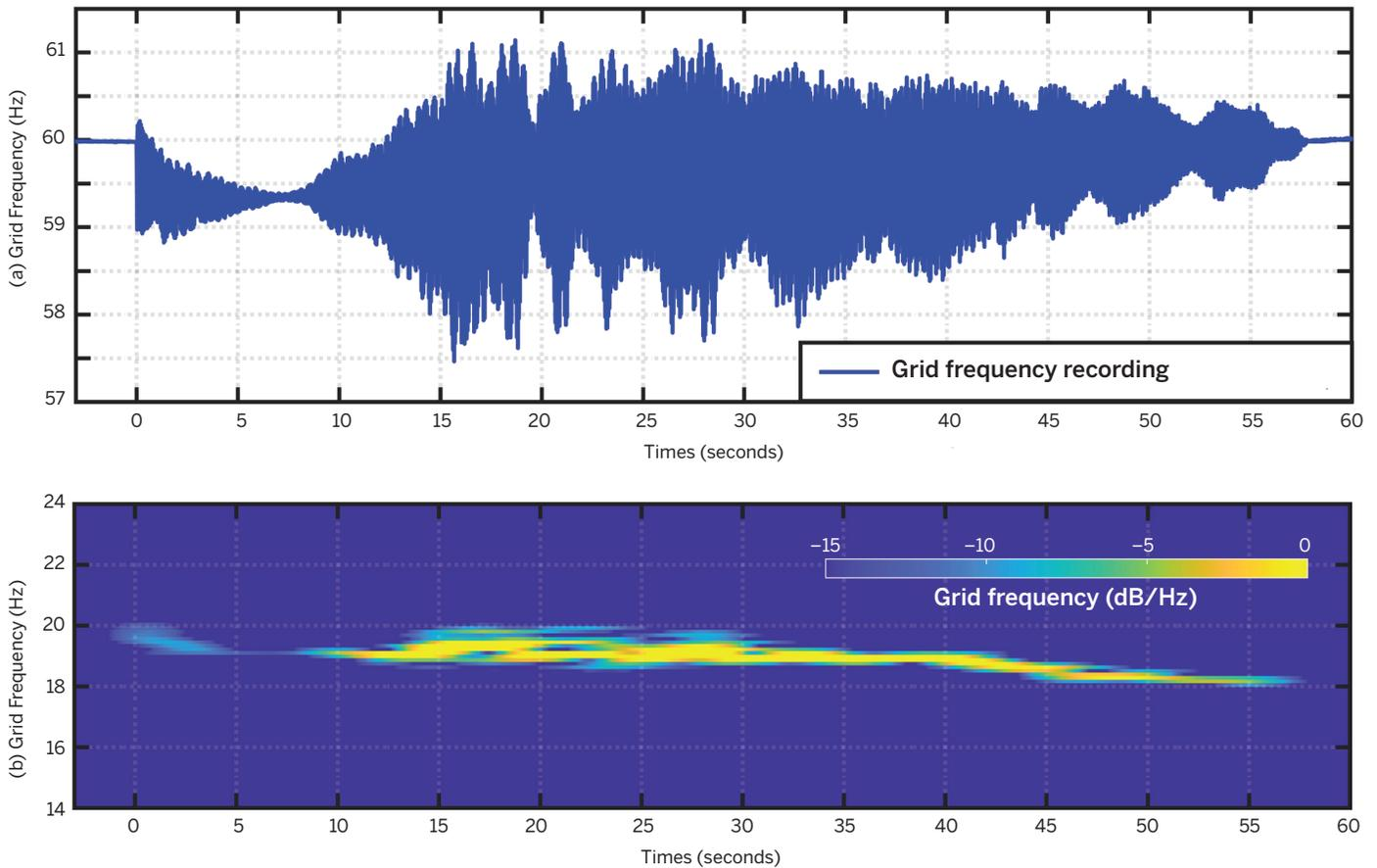
**Example spectrogram of a Kaua'i frequency recording showing 18 to 20 Hz oscillations. (a) Modulation of fundamental frequency. (b) Spectrogram of modulation frequency showing a drift of the modulation frequency from 20 to 18 Hz oscillations over the course of an hour.**
