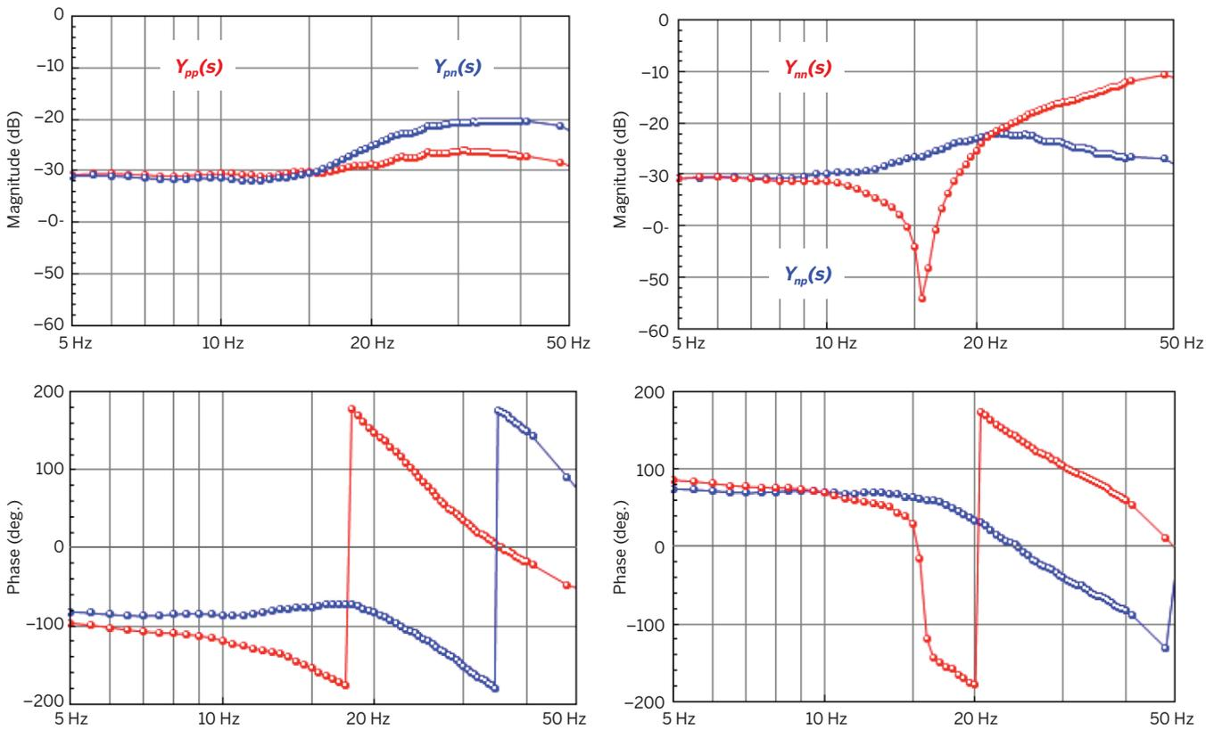
The positive- and negative-sequence dynamic admittances (red traces, left and right, respectively) show sharp negative-sequence resonance at 17 Hz, indicating the IBR will tend to modulate negative sequence at this frequency. Diagonal terms (blue) have little participation at this frequency.
