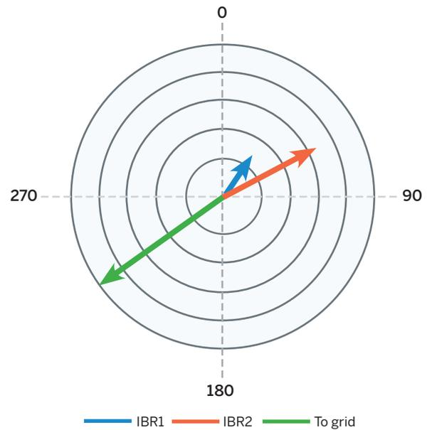
**Polar plot of the currents for one oscillatory mode involving two IBRs. In this case, the two IBRs are largely coherent and are oscillating against the host grid. IBR2 has roughly double the participation of IBR1.**
