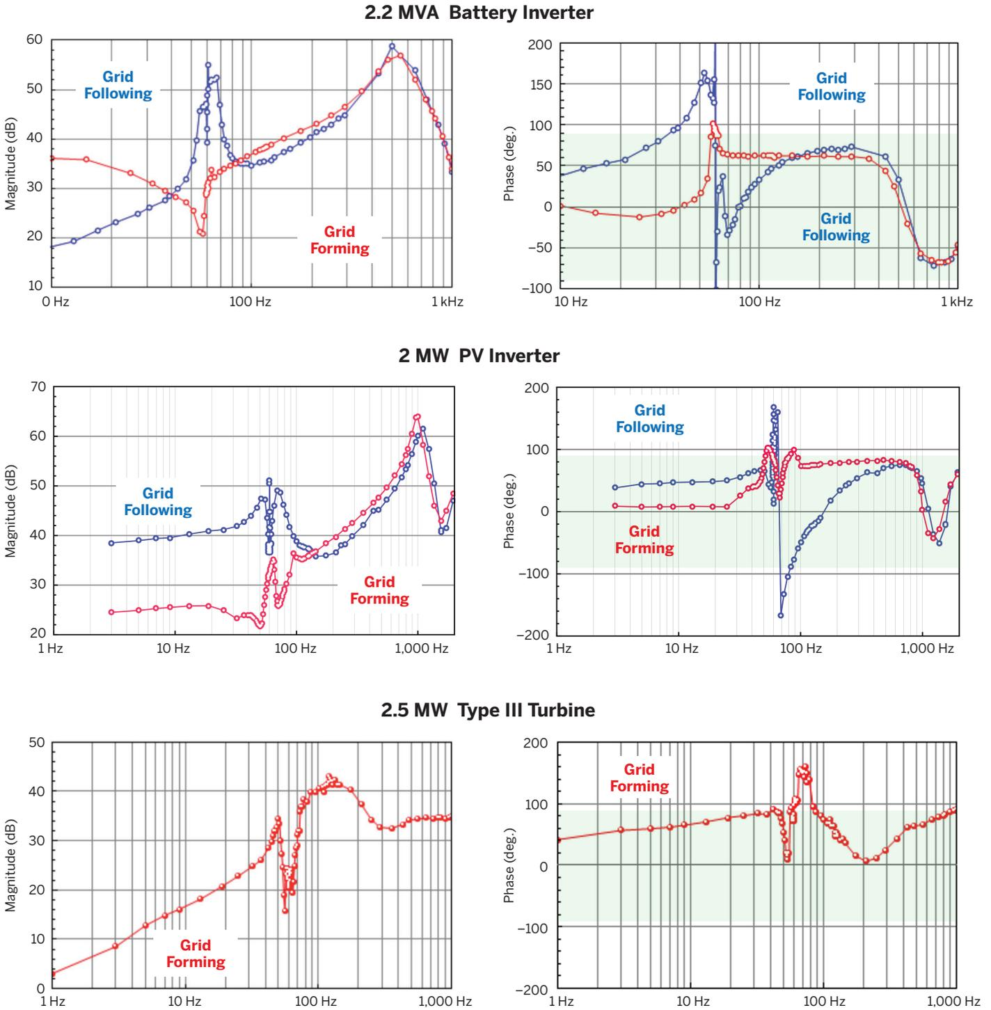
An illustration of the impact of control on the effective impedance of various inverters. This is an effective screening method for stability. When the phase impedance angle is outside  $\pm 90^\circ$ , and the frequency coupling is negligible, the control exhibits negative resistance, which tends to be destabilizing.
