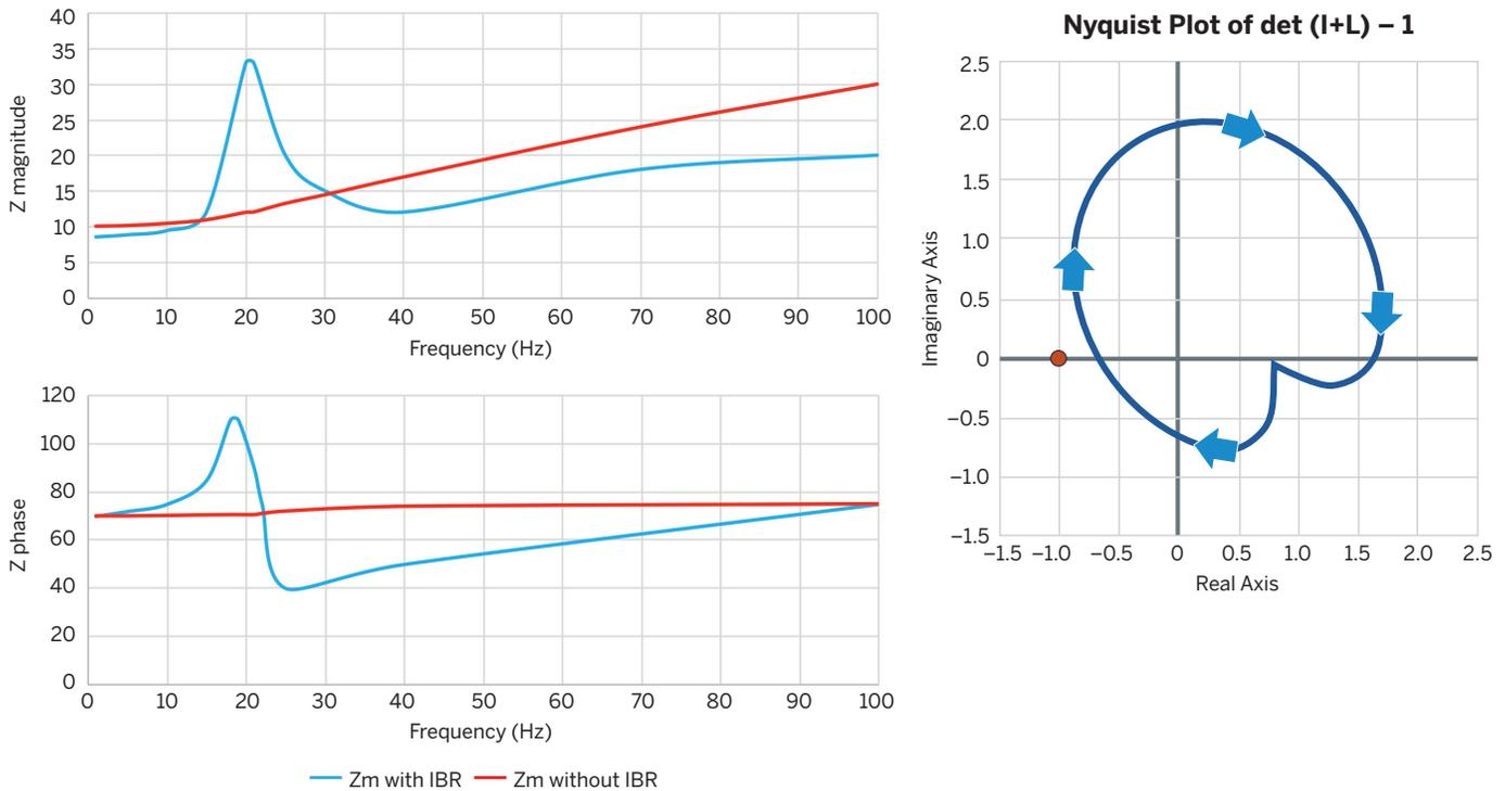
Combined dynamic frequency scans, with and without IBR at the point of connection, showing approximately 19 Hz natural frequency due to the IBR. The corresponding Nyquist plot (on the right) with the IBR, shows that the system is marginally stable at the resonant frequency: it does not encircle  $(-1,0)$ .
