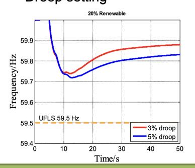
A 3% governor droop can significantly improve the frequency nadir and settling frequency of WECC.
