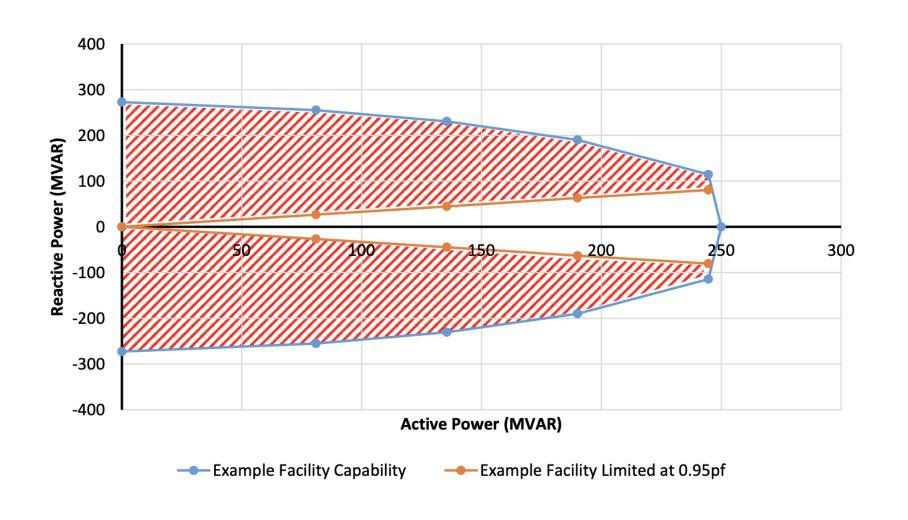
NERC Level 2 Alert data shows 35% of the currently installed IBRs are operating in this limited mode
