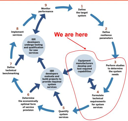
In the proposed process for deploying new GFM capabilities to serve system needs, the outer circle follows steps 1 through 9 as discussed in the text, while the three inner elements show how the nine steps relate to IBR equipment manufacturers and project developers and owners. Steps 1 through 9 are not set in stone and will likely need to be an iterative loop as systems and technologies continue to evolve.
